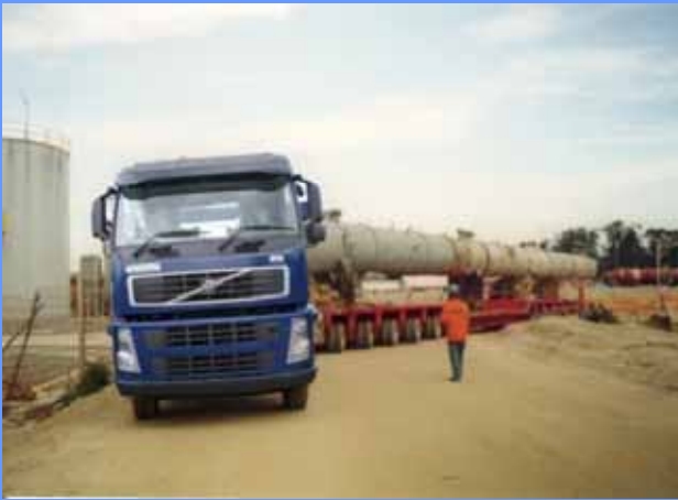
Transportation for Urea Reactor
